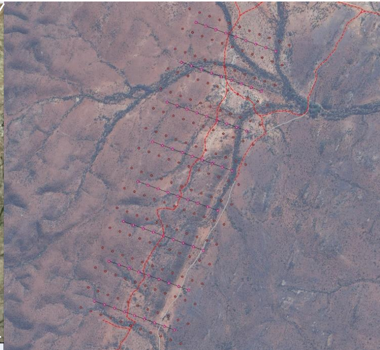
Figure 4 Ground EM traverses over copper mineralisation at Little Gap Well. Data collected in October. Any copper sulphide mineralisation beneath historic pits may be identified as conductive. Pink dots show the location of EM stations. 100m station spacing, 400m line spacing.
