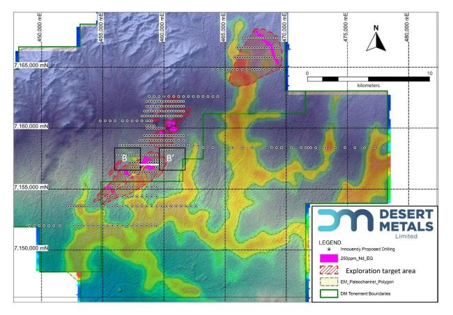
*Figure 9* Planned Innouendy drilling. Background image topography overlain by interpreted paleo channel from airborne EM. Mineralisation has the potential to extent over a large volume.
