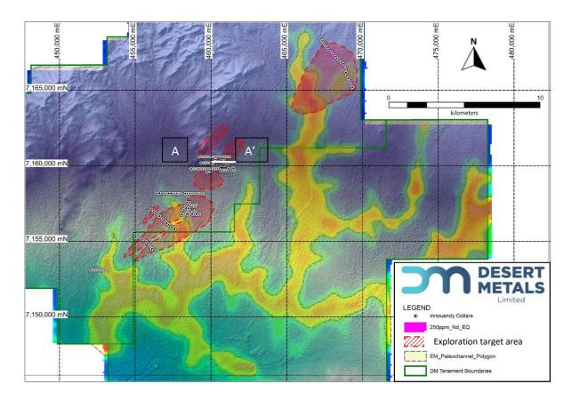
*Figure 6.* Current Innouendy drilling. Background image topography overlain by interpreted paleo channel from airborne EM. Mineralisation has the potential to extend over a large volume.
