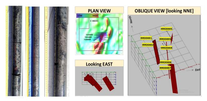
**Figure 1** EM plates and initial drill plan at Irrida Hill. Holes IRRD002, IRRD004 and IRRD005 have now all been drilled and all intersected multiple zones of semi massive to massive sulphide mineralisation. DHEM modelling has identified additional conductors away from these holes.
