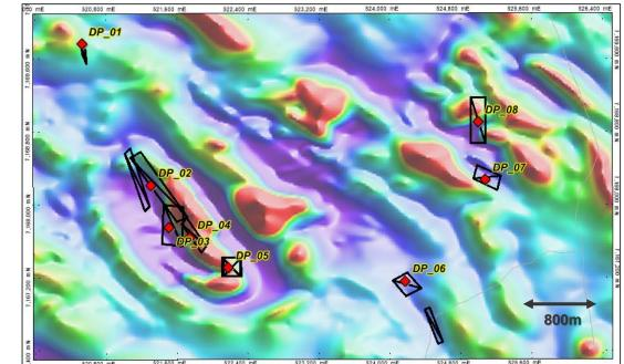
Residual RTP magnetic image below EM modelled plates [projected to surface]. Collars of drill holes planned [subject to refinement] shown.
