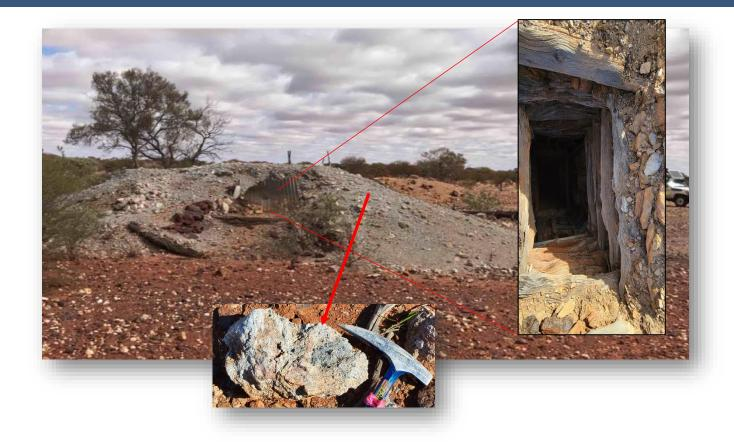
Figure 4. Ajax Mine Historic Working, with inset of mullock material which assayed 17.3g/t Au.
